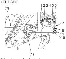
(1) spring pre-load adjuster(2) pin spanner
