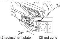
Check the chain wear label when adjusting the chain. If the front edge of the chain adjustment plate (2) enters the red zone (3) on the label after the chain has been adjusted to the proper slack, the chain is excessively worn and must be replaced. The proper slack is:
