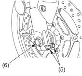
(5) axle pinch bolts(6) front axle bolt
