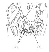
(5) axle pinch bolts(7) front axle shaft
