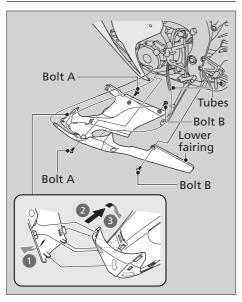
The lower fairing must be removed to adjust the clutch lever freeplay and to change the oil filter.
