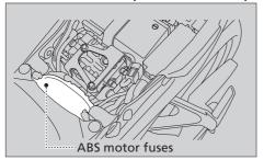
The ABS motor fuses are located on the starter magnetic switch.
