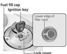
Do not fill with fuel above the lower edge of the filler neck.
