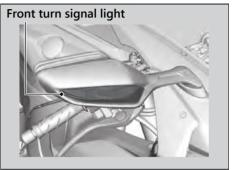
The front turn signal light uses several LEDs. If there is an LED which is not turned on, see your dealer for servicing.
