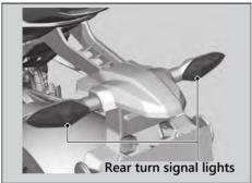
The rear turn signal light uses several LEDs. If there is an LED which is not turned on, see your dealer for servicing.
