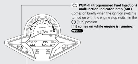
(B) ABS (ant-lock Brake System) indicator (CBR250RA only)
