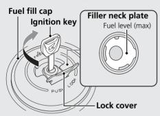
Do not fill with fuel above the plate. **Fuel type:** Unleaded gasoline only **Recommended fuel octane number:**Pump Octane Number (PON) 86 or higher. **Tank capacity:** 3.43 US gal (13.0 liters)
