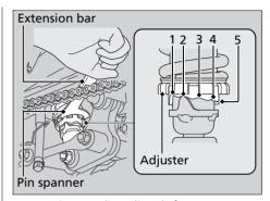
Attempting to adjust directly from 1 to 5 or 5 to 1 may damage the shock absorber.
