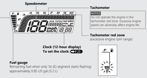
If the fuel gauge indicator flashes in a repeat pattern or turns off: P.94
