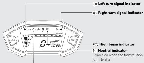
PGM-FI (Programmed Fuel Injection) malfunction indicator lamp (MIL)
