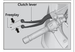
Check the clutch cable for kinks or signs of wear. If necessary have it replaced by your dealer.
