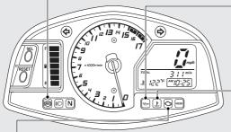
Low oil pressure indicator Comes on when the ignition switch is turned to the ON position. Goes off when the engine starts. If it comes on while engine is running: P.83
