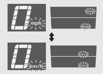
Press the SET button. The speed and mileage unit is set, and then the display moves to the changing of the coolant temperature gauge unit.
