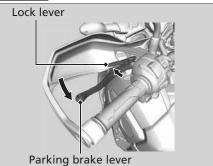
Place your motorcycle on a firm, level surface. Stop the engine and push your motorcycle while set the parking brake to check the efficacy of the parking brake.
