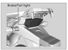
The brake and tail light uses several LEDs. If there is a LED which is not turned on, see your dealer for servicing.
