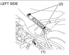
(1) swingarm bushing(2) shock absorber attachment points
