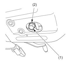
(1) oil drain bolt(2) sealing washer
