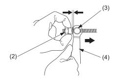
(2) adjusting nut (3) brake arm pin
