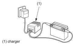
Be sure to read the information that came with your battery charger and follow the instructions on the battery. Improper charging may damage the battery. We recommend using a charger (1) designed specifically for your Honda, which can be purchased from your dealer. These units can be left connected for long periods without risking damage to the battery. However, do not intentionally leave the charger connected longer than the time period recommended in the charger's instructions.
