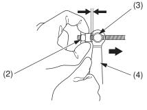
(2) adjusting nut(3) brake arm pin
