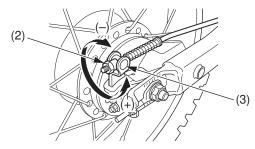
(2) adjusting nut(3) brake arm pin
