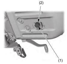
(1) oil drain bolt(2) sealing washer
