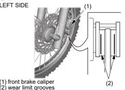
Check the wear limit grooves (2) in each pad. If either pad is worn to the groove, replace both pads as a set. See your dealer for this service.
