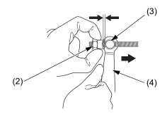
(2) adjusting nut (3) brake arm pin
