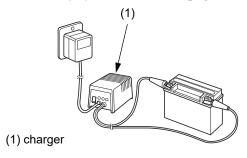
Be sure to read the information that came with your battery charger and follow the instructions on the battery. Improper charging may damage the battery. We recommend using a charger (1) designed specifically for your Honda, which can be purchased from your dealer. These units can be left connected for long periods without risking damage to the battery. However, do not intentionally leave the charger connected longer than the time period recommended in the charger's instructions.
