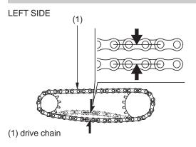
1. Check slack in the lower drive chain (1) run midway between the sprockets. Drive chain slack should allow the following vertical movement by hand:
