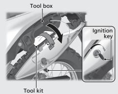
Insert the ignition key and turn it clockwise to open the tool box.
