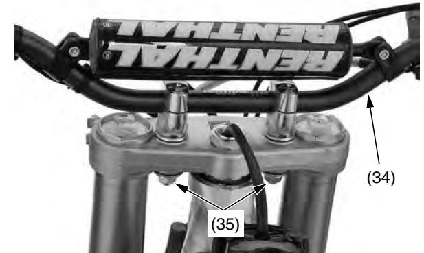
(34) handlebar (35) mounting rubbers, washers and handlebar lower holder nuts
