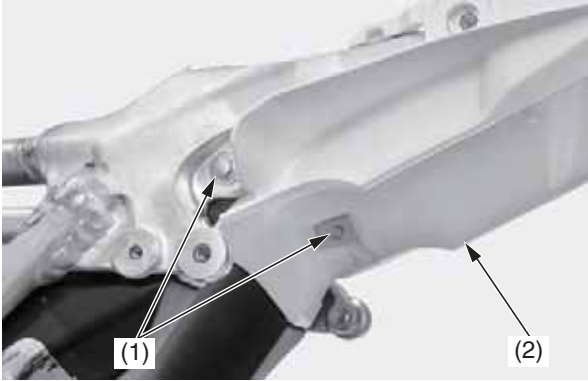
(1) rear fender mounting bolts and nuts (2) rear fender
