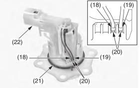
(18) red wire terminal (19) black wire terminal (21) O-ring (new) (22) fuel pump unit
