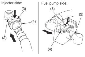
(2) fuel joint(3) slide retainer(4) connector housing
