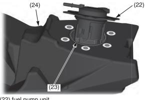
(22) fuel pump unit (23) O-ring (new) (24) fuel tank
