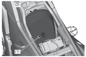
(1) air cleaner retaining bolt(2) air cleaner assembly
