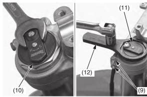
(9) fork bridge upper pinch bolts(10) fork bolt assembly(11) fork damper assembly(12) lock nut wrench
