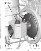
(15) front axle nut(16) axle pinch bolts
