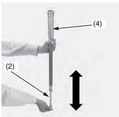
(2) fork damper piston rod (4) fork damper assembly
