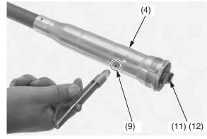
(4) fork damper assembly(9) oil hole(11) air pressure release screws(12) O-rings (new)
