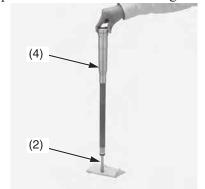
(2) fork damper piston rod(4) fork damper assembly
