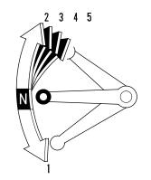
Your CRF has five forward gears in a one-down, four-up shift pattern.
