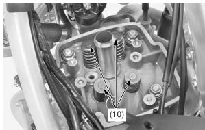
(9) intake valve lifters (10) shims
