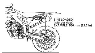
Example: Unloaded = 600 mm (23.6 in) -Loaded = 550 mm (21.7 in) Sag = 50 mm (2.0 in) (Without Rider)
