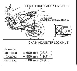
Calculate the *race sag* dimension. To do this, subtract the *loaded with rider* dimension (step 3) from the *unloaded* dimension (step 2). Standard Race Sag: 100 mm (3.9 in)
