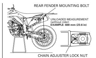
3. Measure the *loaded with rider* dimension. Remove the workstand. With two helpers available, sit as far forward as possible on your CRF's seat, wearing your riding apparel. Ask one helper to steady your CRF perfectly upright so you can put both feet on the pegs. Bounce your weight on the seat a couple of times to help the suspension overcome any situation and settle to a good reference point.
