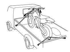
To secure your CRF, brace the front wheel against the front of the truck bed or trailer rail. Attach the lower ends of two straps to the tiedown hooks on your CRF. Attach the upper ends of the straps to the handlebar (one on the right side, the other on the left), close to the fork.
