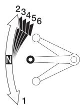
Your CRF has 6 forward gears in a one-down, fiveup shift pattern.
