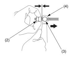
(2) adjusting nut (3) brake arm pin
