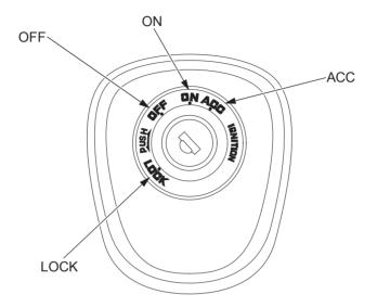
The ignition switch is used for starting and stopping the engine (page 55) and to lock the steering for theft prevention (page 65). Insert the key and turn it to the right for the ON and ACC (accessory) positions.
