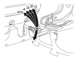
Your motorcycle has five forward gears in a one-down, four-up shift pattern which is coordinated with a hydraulically actuated clutch system.
