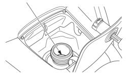
Add fuel until the level reaches the bottom of the filler neck.
