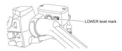
Check that the fluid level is above the LOWER level mark. If the fluid level is below the LOWER level mark, it indicates fluid leakage. See your dealer for repair.
