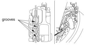
Always inspect both pads in both the right and left front brake calipers.
